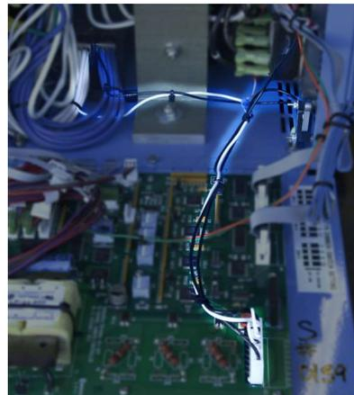
This tab's function is to cut off power to the processor whenever the dimmer door is open as a safety precaution. However, if the trip switch is not securely fastened on both ends, whether it be the crimp on the black lead to the 9 pin power input or the lug connecting to the top of the trip switch, the power will not be able to be supplied to the processor as the circuit is remaining open.
